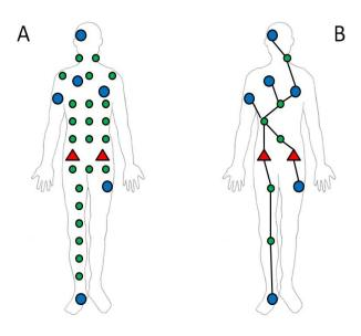
Figure 3: The figure shows the potential topology of a BAN using relay nodes, represented as circle of smaller sizes, and the realized topology, where just a subset of relays has been activated.
