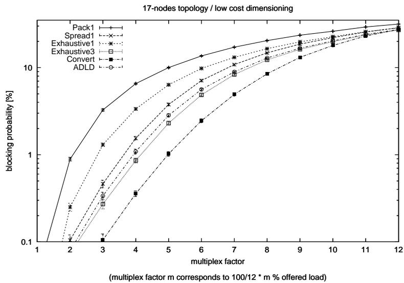
FIGURE 3. Blocking probability of the algorithms on the 17-nodes network with low cost dimensioning
