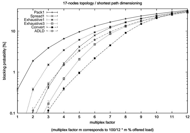
FIGURE 2. Blocking probability of the algorithms on the 17-nodes network with shortest-path dimensioning
