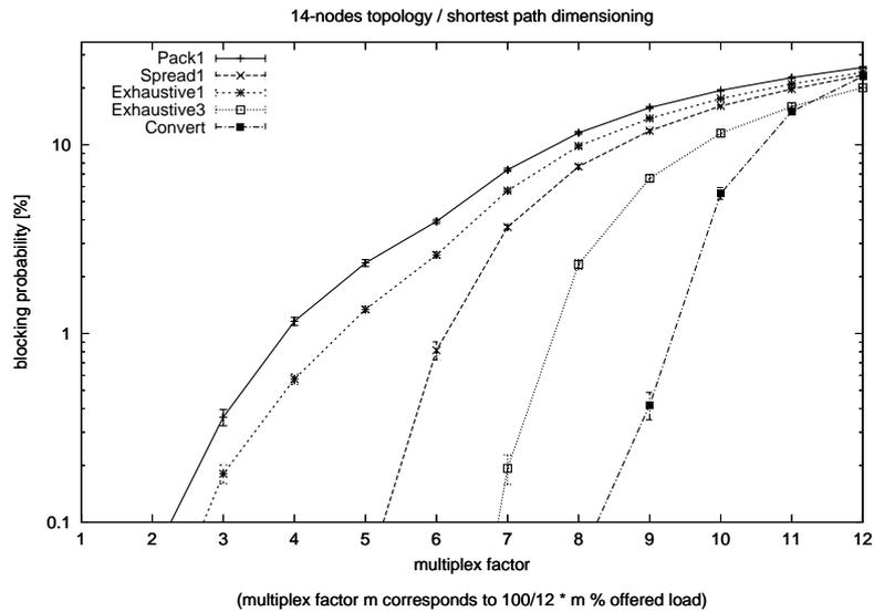
FIGURE 4. Blocking probability of the algorithms on the 14-nodes network with shortest-path dimensioning
