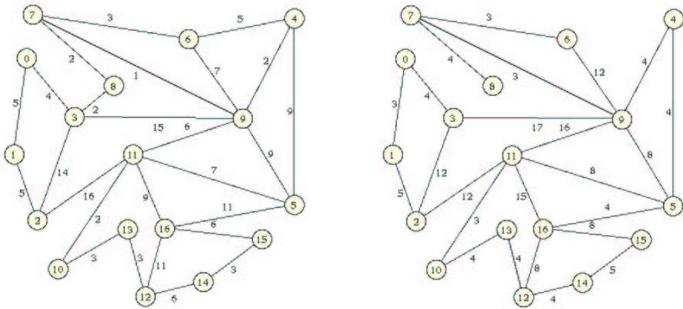
FIGURE 11. The 17-nodes network with shortest path and with low cost dimensioning
